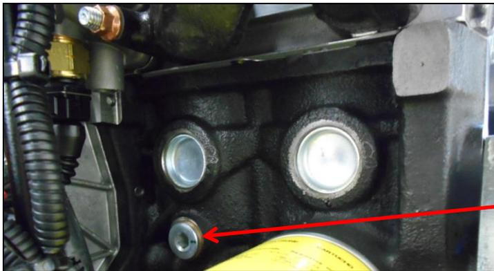
Engine Coolant Drain Plug
