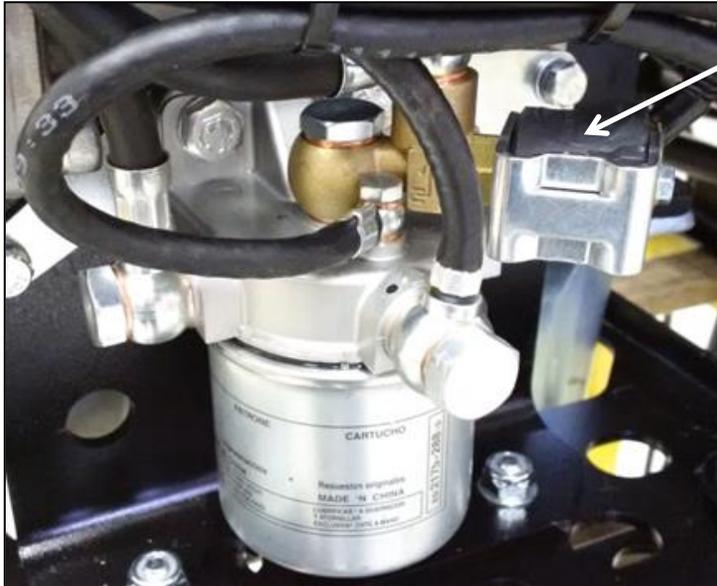
**Fuel Shut-Off Solenoid****Removal of the Fuel Solenoid**
