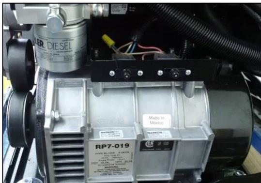
To clean generator: remove plastic end cap by unscrewing the two (2) bolts at the back.
