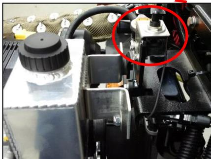
The safety cover switch (See Figure 0-1) is designed to prevent the RigMaster Power APU from starting when the engine cover is loose or has been removed. When the cover is down, the switch is in the closed position. When the cover is open or loose, the switch is in the open position. The switch is located at the very top of the unit enclosure on the surge tank bracket.
