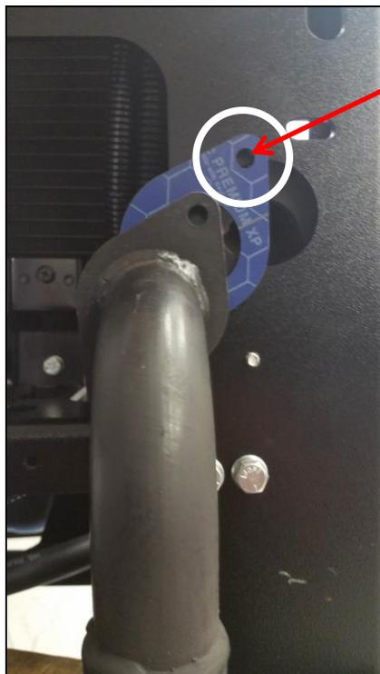
The muffler flange mounts to 2 holes in the Bulkhead with Gasket (only 1 hole is shown) (See Figure 8-4)
