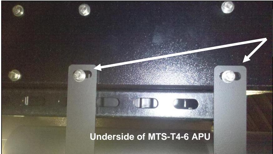
Muffler Lower Mounting Tabs (See Figure 8-6) are bolted to the bottom of the Left-side APU Frame rail.
