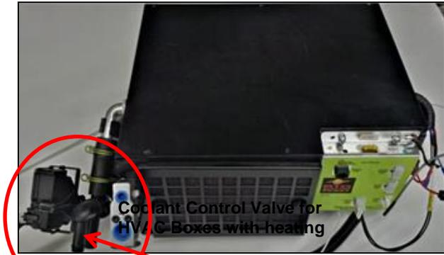
**Coolant Control Valve for HVAC Box with Heat**
