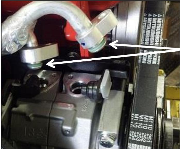
Lubricate O-rings and install A/C hose fittings into the compressor ports.
