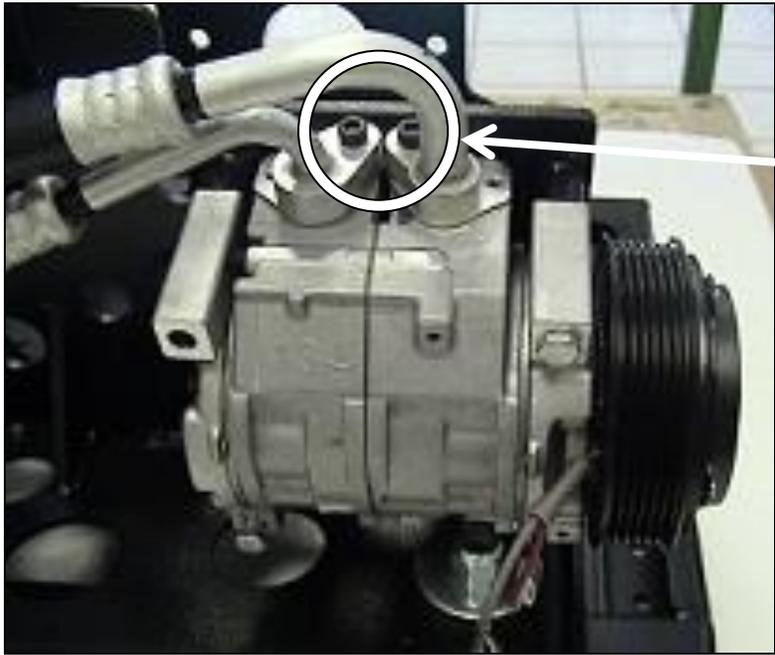
Torque the A/C hose clamp bolts to 7 ft/lbs.
