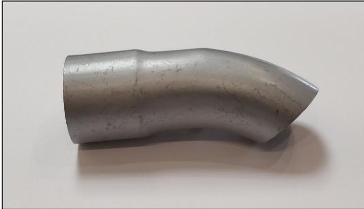
The exhaust tip included in the packaging of a new APU is not a mandatory component in this exhaust system. It must be removed to add an extension tail pipe. (See NOTE above). When installing this component use a 1½" pipe clamp to ensure that the connection stays tight on the muffler.
