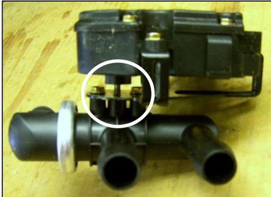
**Control Valve Motor Shaft**
