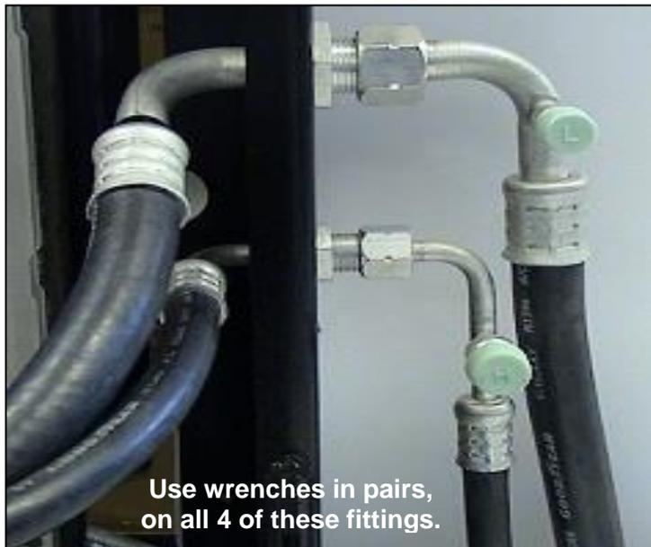
5. After installation, deflate the cab air suspension and inspect hoses for potential clearance problems. To avoid hose failures from damage, A/C hoses should not be under twisting or flexing stresses after installation.
