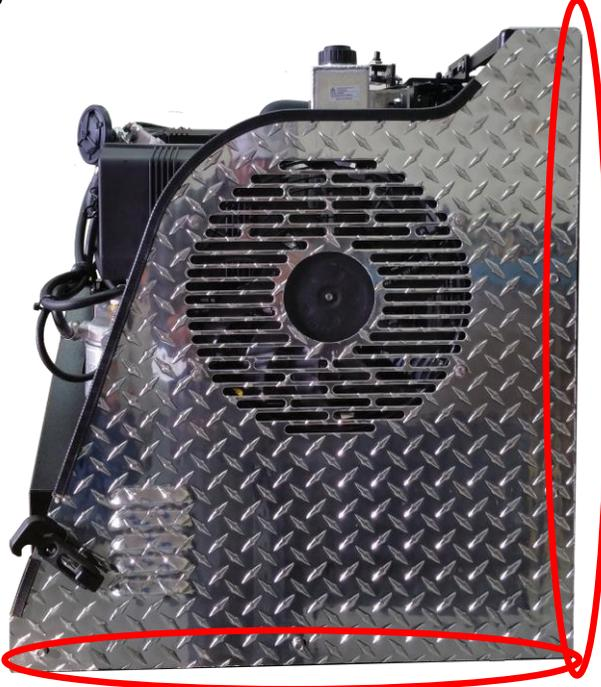
The APU Side Panels are mounted to the APU Frame with 1/4"-20 Bolts (x 12)
